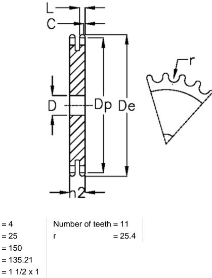
De = 150Dp = 135.21For chain size =  $1 \frac{1}{2} \times 1$ For chain type = 24 B-2h2 = 72L = 23.6
